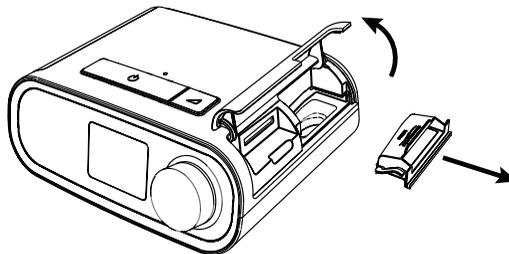
2. If applicable, place a dry, reusable blue pollen filter (1) on top of a new, optional disposable light-blue ultra-fine filter (2) and firmly snap them together.
