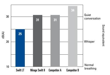
Testing per ISO 3744: 1994 Acoustics determination of sound power levels of noise using pressure at 10 cm  $\rm H_2O.$
